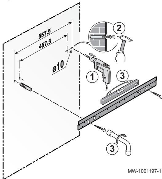
1. Drill 2 holes with a diameter of 6 mm.
