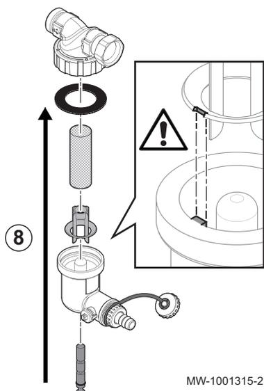
8. Refit the sludge collector.
