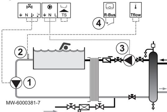
1. Connect the swimming pool's secondary pump to the three-way valve terminal block for the **CIRCA1**, **CIRCB1** or **CIRCC1** circuit.
