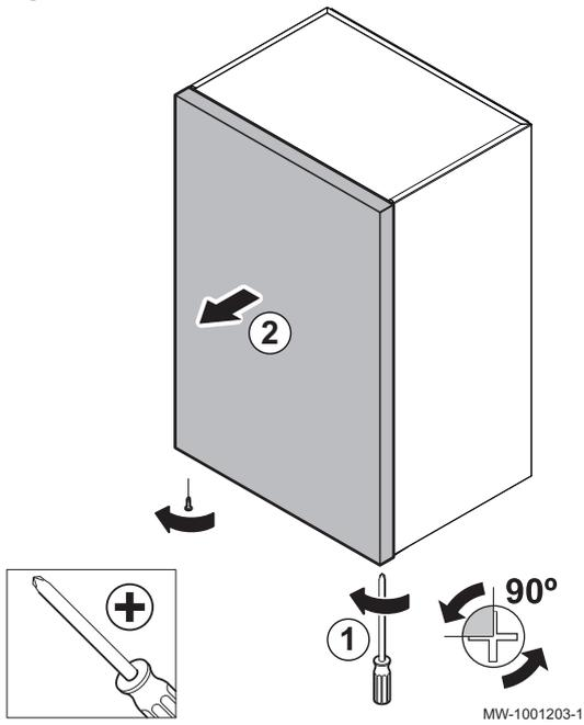
1. Unscrew the two screws under the front panel by a quarter turn.
