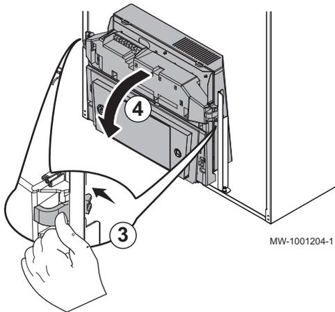
3. Open the holding clips located on the sides.
