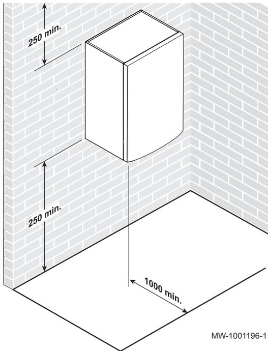
Allow sufficient space around the heat pump indoor module to ensure adequate access and facilitate maintenance.
