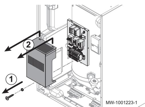
1. Remove the retaining screw.
